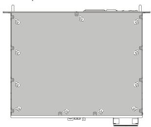
☐ Remove the four screws on the dummy panel of the **VXR-9000**, then remove the dummy panel from the **VXR-9000**.
